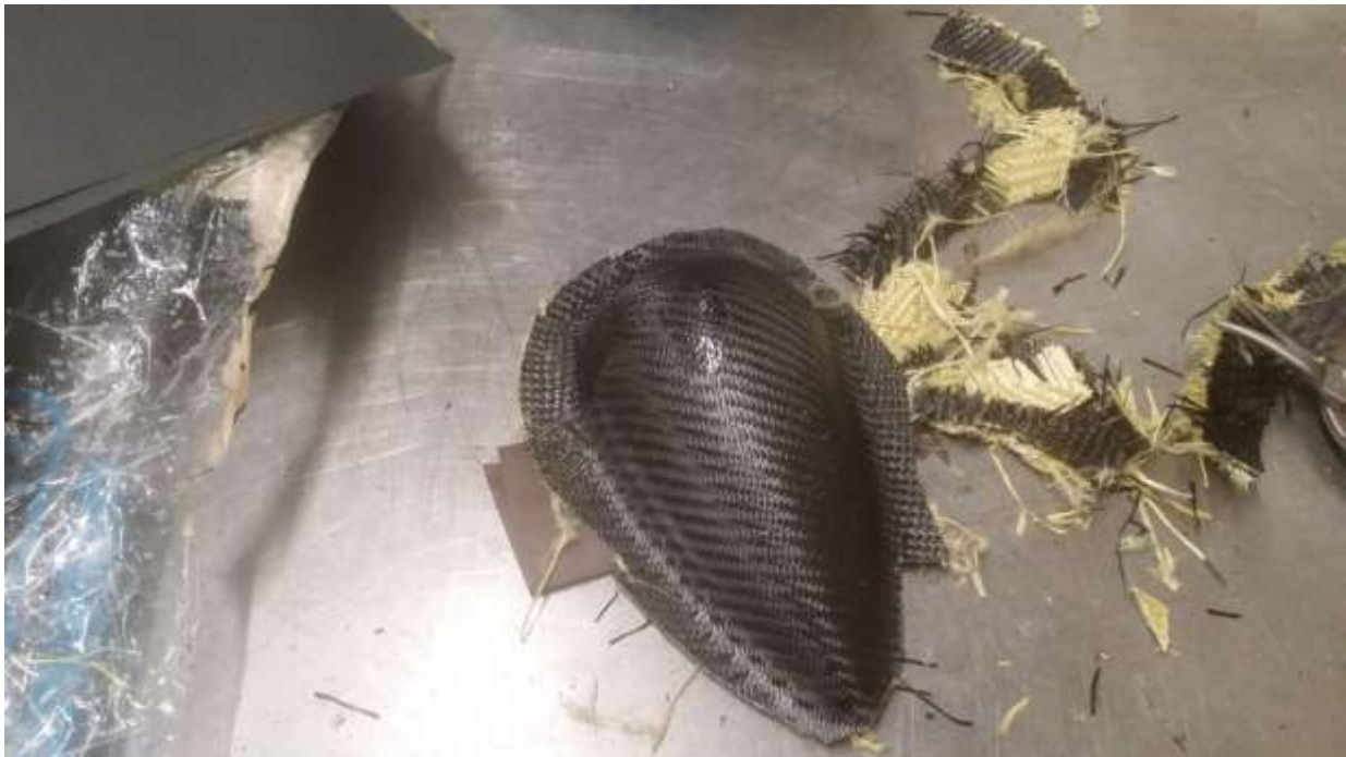
Figure 10 Trimming Excess of Hardened Piece - J.King 2014
