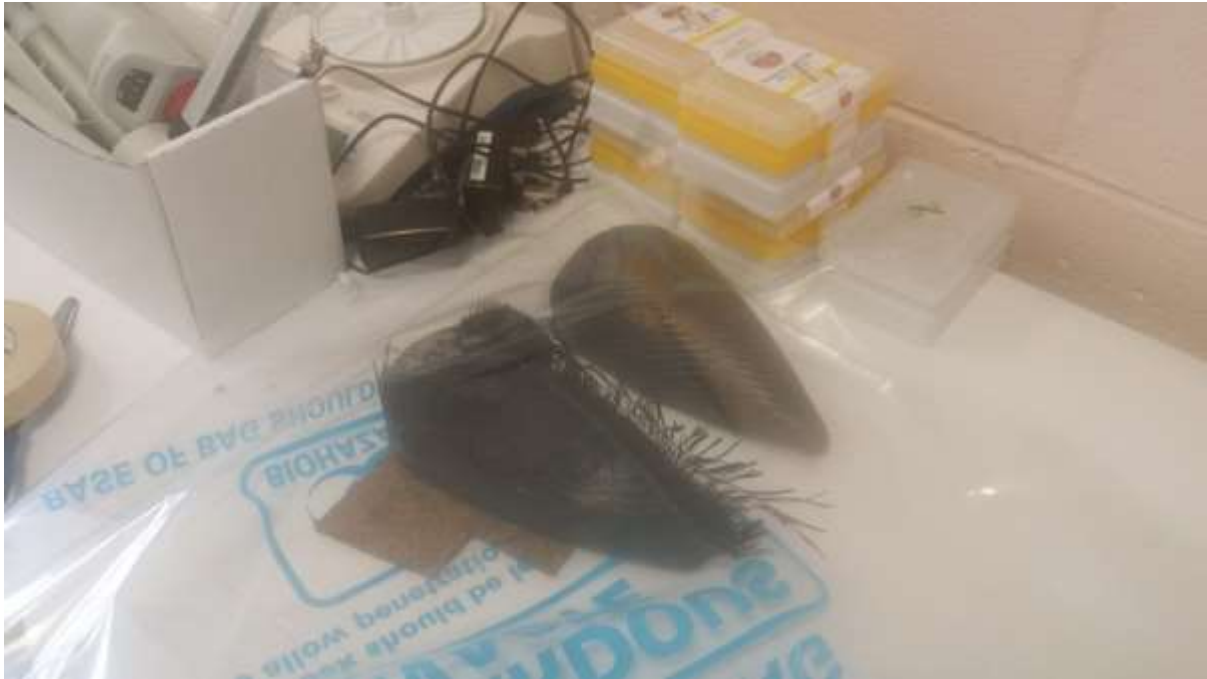
Figure 9 Pieces ready for Autoclave in Vacuum Bag - J.King 2014
