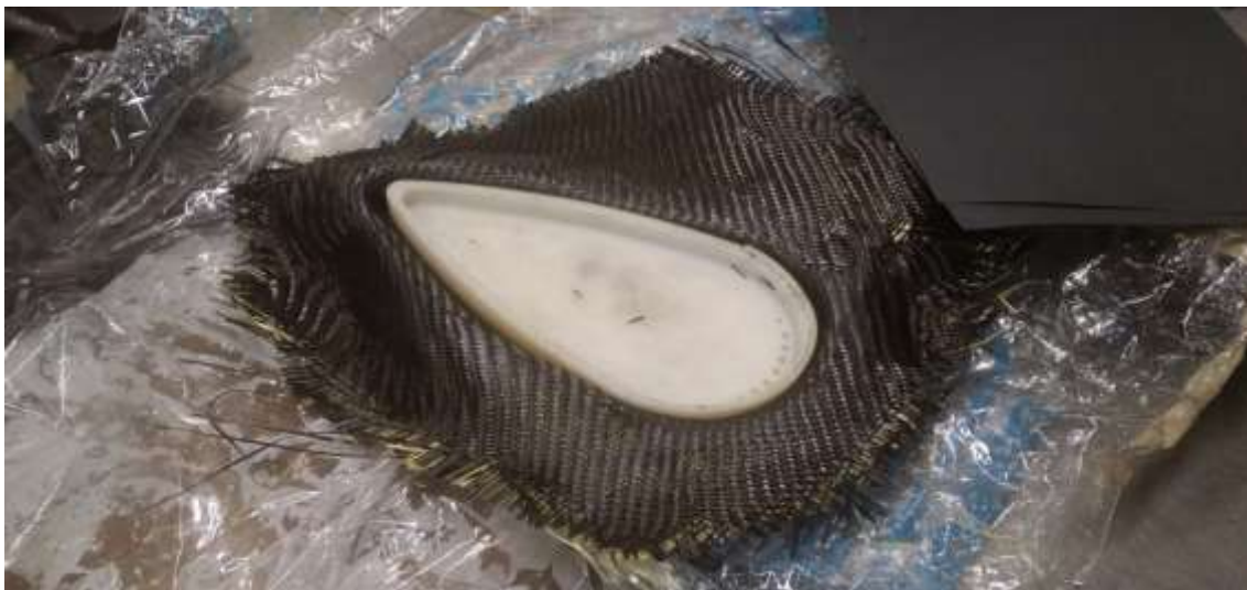
Figure 8 Carbon Fibre and Kevlar Application on Developed Mould - J.King 2014
