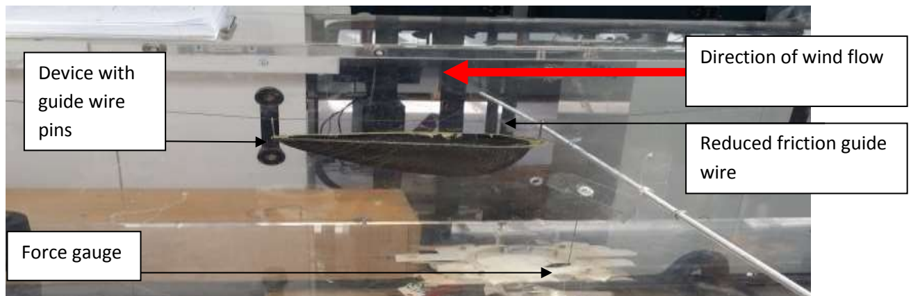
Figure 16 Medi-Pod™ Prototype Wind Tunnel Aerodynamic Optimisation Experimental Test Set Up - J.King 2014
