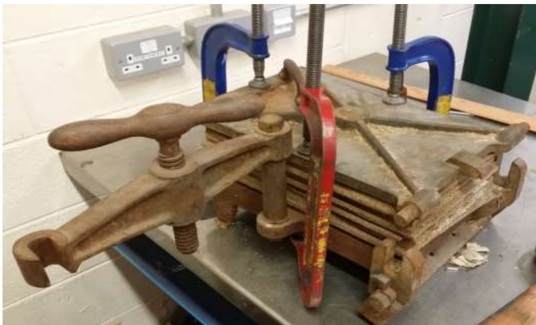
Figure 12 Viner Pressing the Layers of Cork - J.King 2014
